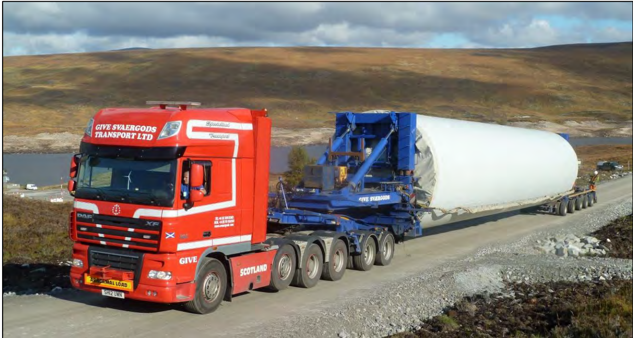
Figure 3: Base Tower Trailer
